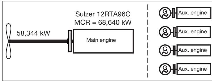
Fig. 13: Schematic of the conventional propulsion plant – the basis.
