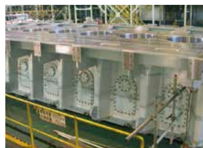
Fig. 3: Welded cylinder frame for a 7S65ME-C
