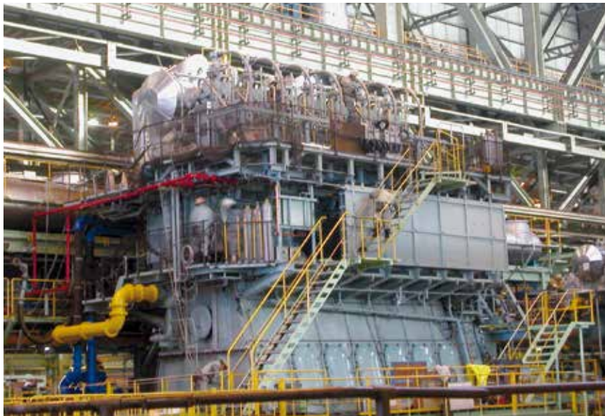
Fig. 1: Shop test of 7S65ME-C engine at Hitachi in March 2006
