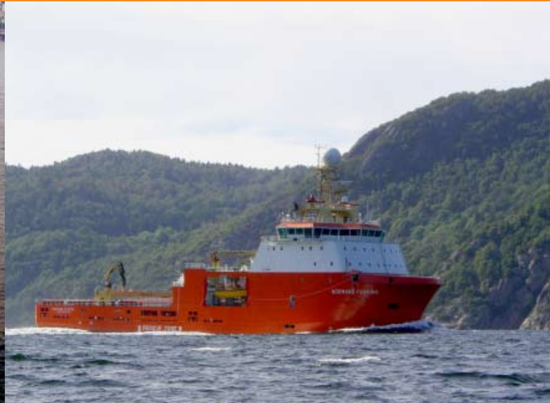
The anchor handling tug supply vessel Normand Ferking is equipped with two Wärtsilä TCH270-PS58SDC63 gears.
