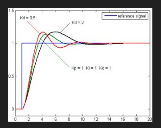
Response to Unit step of a D controller
