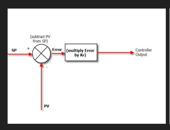
In Proportional Only mode, the controller simply multiplies the Error by the Proportional Gain (Kp) to get the controller output.
