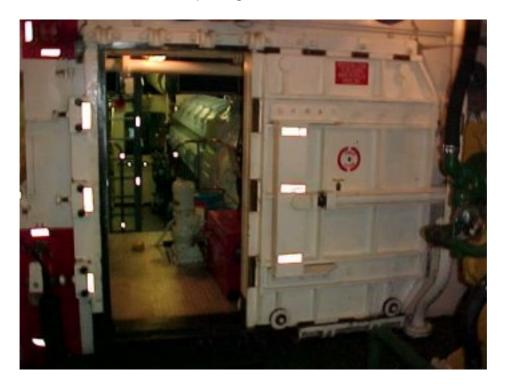
The crew routinely passed through the watertight doors without fully opening them when the doors were in the local-control mode. This practice was probably also followed when the doors were in the remote-close mode. It is possible that the victim tried to pass through the door before it was fully open, and for some reason (such as releasing the handle) it began closing and trapped him.
