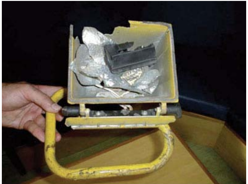
Figure 2: remains of the non-intrinsically safe halogen lamp that caused the explosion
