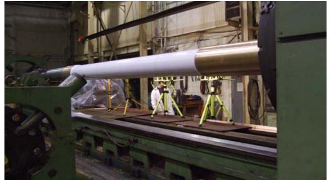
Figure 5. Thor-Coat shaft coating applied to shafts.
