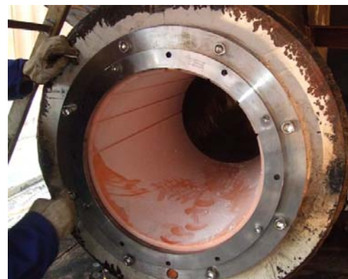
Figure 2. Retaining ring fitted to COMPAC bearing carrier
