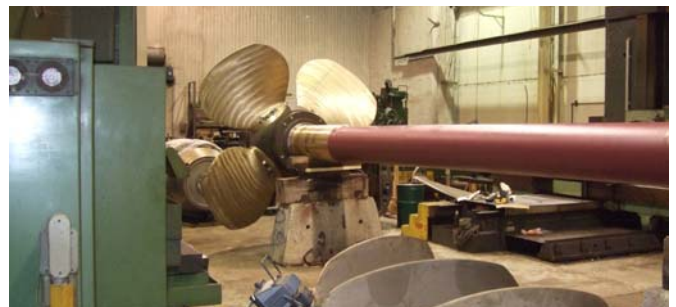
Figure 6. Shaft coated with a tin-free anti-fouling paint.
