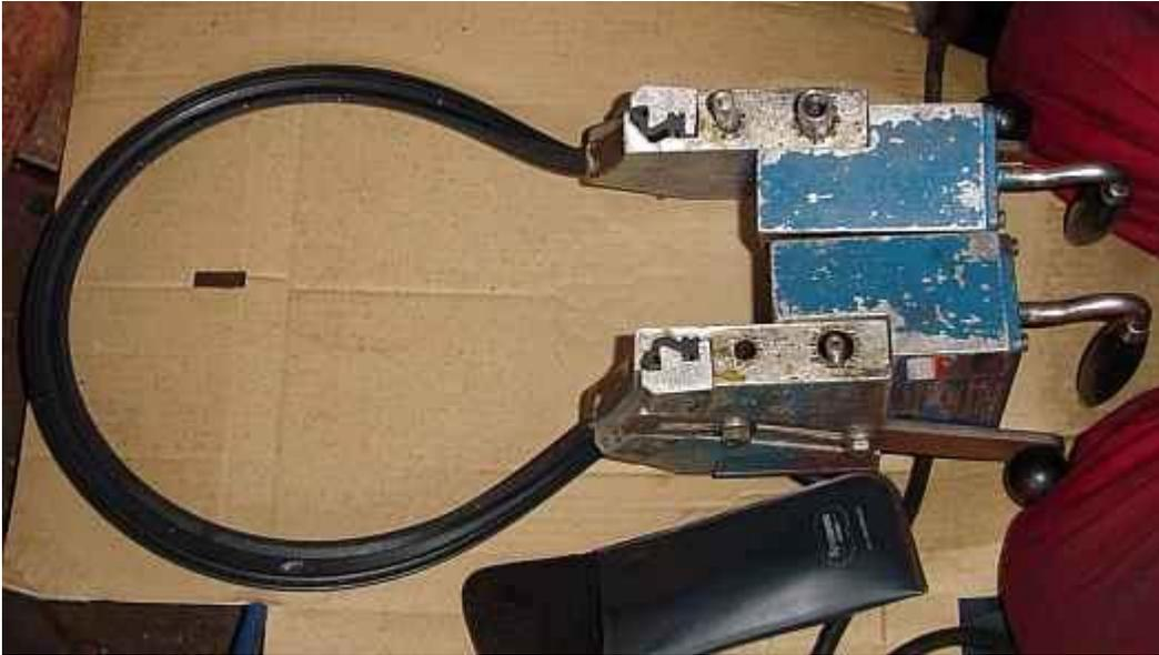
The vulcanising machine is then set up off the shaft and the position of the seal checked.
