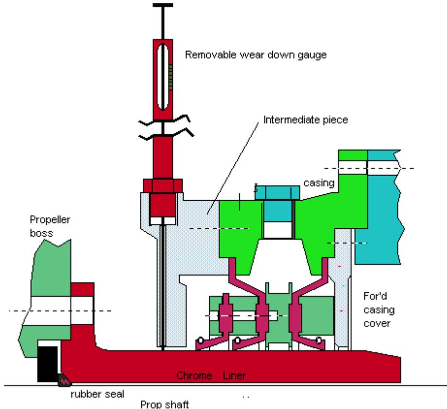
A very common arrangement for oil lubricated stern tube bearings. A simplex seal arrangement is fitted to both inner and outer ends.
