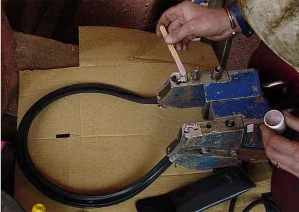
The vulcanising machine is then fitted to the shaft and connected to an electrical supply. A heater within the machine heats the seal to a predetermined temperature for a set time determined by ambient temperature, material type etc.
