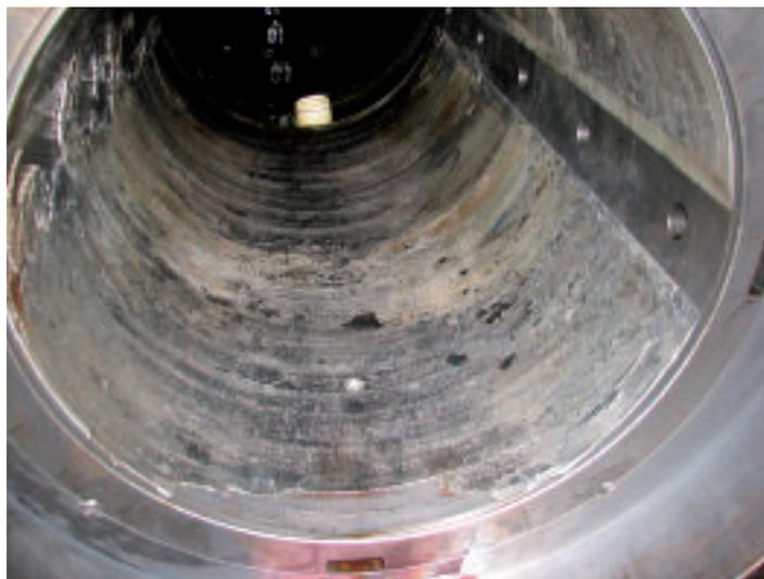
Fig. 2: Condition of white metal bearing found in the aft stern tube bearing.
