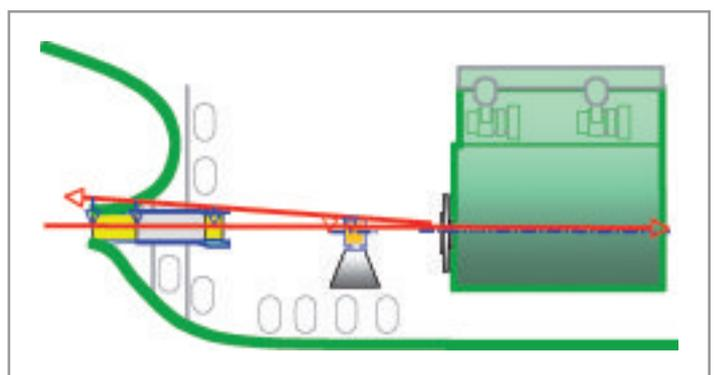
**Fig. A1: Reference line from stern tube to engine and from engine to stern tube.**
