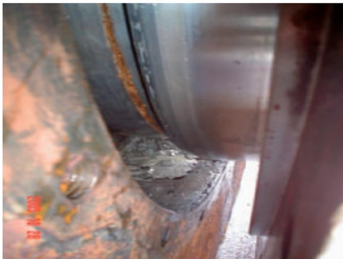
Fig. 1: Pieces of white metal found in the aft stern tube bearing after removal of seal.
