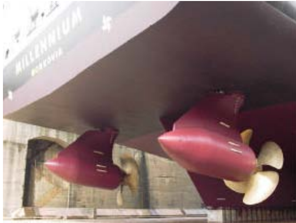
AZIPOD facing Forward in Twin Screw Vessel
