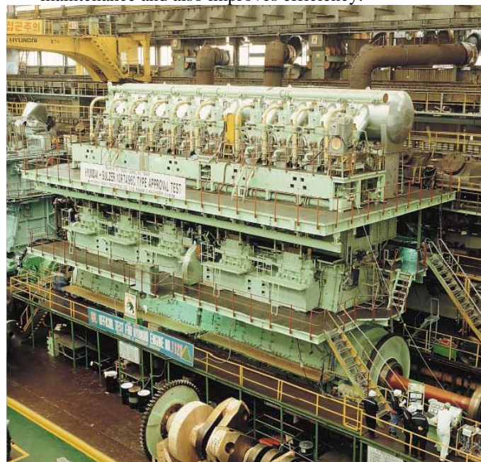
Large engine use to turn propeller in Conventional propulsion
